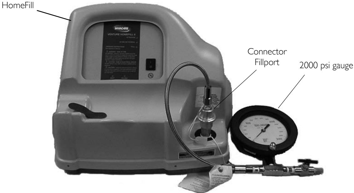
FIGURE 13.3 HomeFill 2000 psi Switch/P.C.B. Shut Down Test
